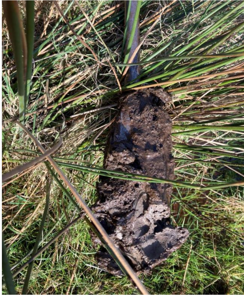
3298/HLA/P5: Auger sample of grey, sticky clay
